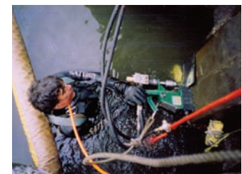
HB-4400 – for Underwater Hydraulic power ø 2-1/16" cutter capacity ø 1/2" twist drill For marine, construction and underwater applications
