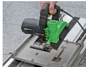
fixing of the saw without any tool
